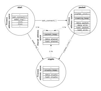
Figure 3: The ELFbac policy for CVE-2016-0777. Three states (start, packet, and crypto) represent the various phases of program execution. Each state is associated with a private and shared process memory layout. This dissection allows ELFbac to enforce separation between crypto-related memory and network traffic.
