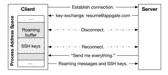
Figure 1: The information leak within OpenSSH. A malicious server convinces a client to return sensitive data upon a roaming reconnect.
