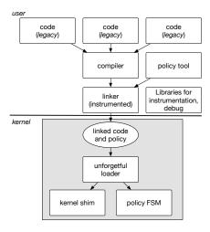
Figure 2: The ELFbac architecture. Legacy code is compiled and linked with an ELFbac policy. During runtime, an ELFbac-aware loader and kernel shim enforce the policy via FSM state transitions.
